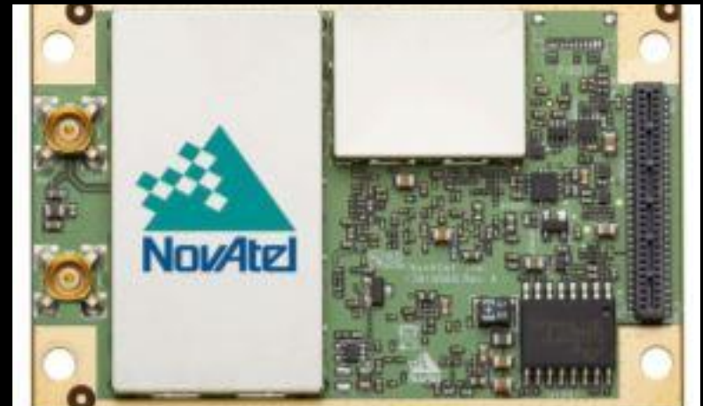
GPS Receiver: Novatel OEM7720
