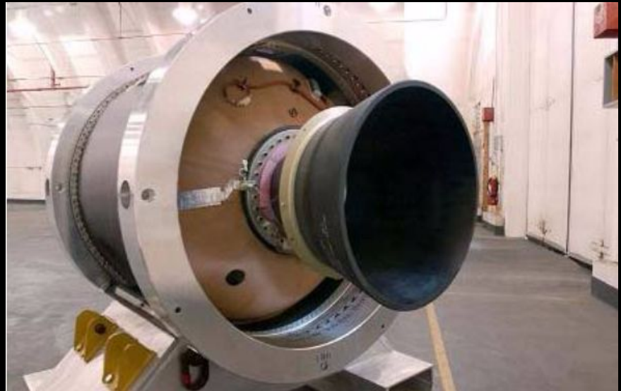
Orion 38 - High performance third stage motor
